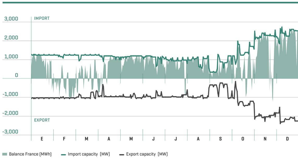
The bringing into full service of the new Santa Llogaia-Baixas interconnection doubled the exchange capacity between Spain and France in the last months of 2015
