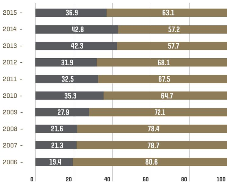
■ Renewable: hydro, wind, solar photovoltaic, solar thermal and other renewables. Does not include pumped storage generation.
