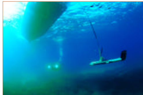
Thorough search of the Santa Ponsa Bay by means of imaging sonar to detect the position of posidonia meadows.
