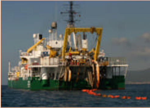
The Skagerrak , Norwegian vessel belonging to Nexans designed specially for undersea cable-laying.
