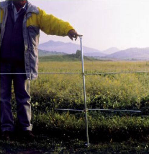
Anti-nesting devices Consisting of differing numbers of rods (with a length of 60 cm, and thickness of 2 cm) and smaller rods (with a length of 1 m, and thickness of 6 mm) laid out in different directions
